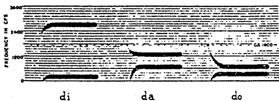
FIG. 1. Spectrographic patterns that produce /di/, /da/, and /do/. The dashed lines are extrapolations to the /d/ locus at 1800 cps.
