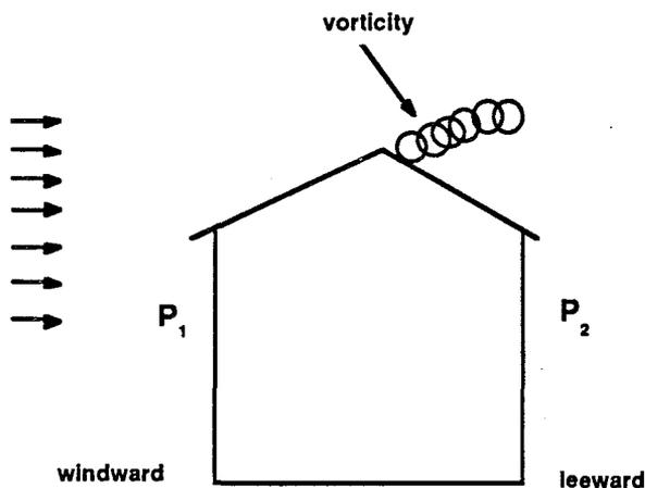
Figure 5. Total pressure on the windward side > total pressure on the leeward side, so that the air pressures are related  $P_1 > P_2$ .
